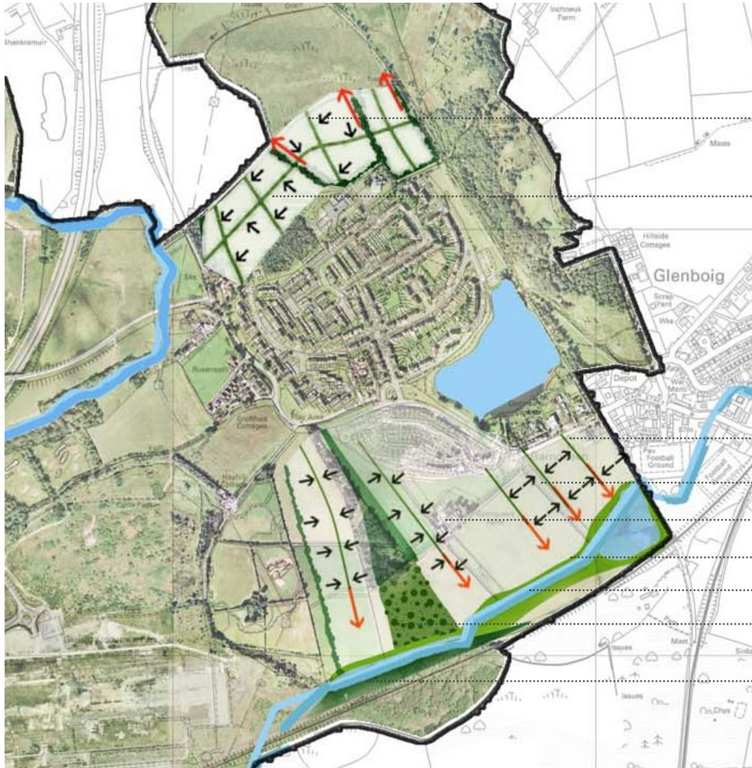
planted swale network, forming 'green street' layout and conveyance routes: integrates habitat and sustainable urban drainage networks whilst providing new pedestrian access routes
